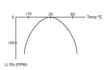
To calculate the frequency stability the parabolic curvature constant (K) is needed. For calculating the stability at  $45^{\circ}\text{C}$ ?
