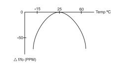
To calculate the frequency stability the parabolic curvature constant (K) is needed. Example: Calculating the stability at  $45^{\circ}$ C
